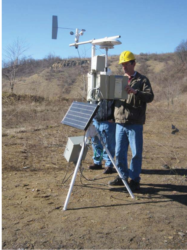
Figure 31. Meteorological monitoring equipment at mine site.
