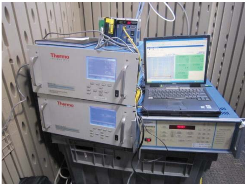
Figure 32. Continuous gas analyzers with calibrator and datalogger.
