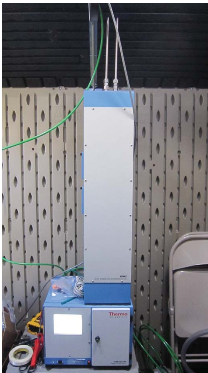
Figure 33. TEOM used to continuously measure PM_{10} and PM_{2.5} at residence.
