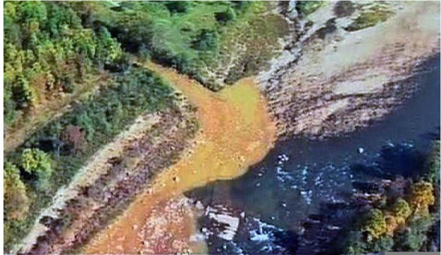
Photo 1. An aerial shot of AMD entering the Cheat River main stem from Muddy Creek during the first and most devastating mine blowout.
